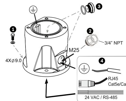
1. Attach DCA to mounting location using user-supplied hardware (item 1). (Bosch recommends stainless steel bolts and washers.) Attach user-supplied conduit or glands to side or bottom hole. If applicable, use the supplied conduit adapter (male M25 to female 3/4 in. NPT) (item 2) if needed. Plug unused hole (item 3). Route cables into DCA (item 4).
