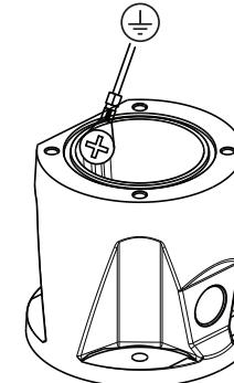
6. Screw green GND wire from camera base to ground hole on inside wall of DCA. If DCA is not mounted to earth grounded surface, attach user-supplied grounded wire (item 4 in step 1) to same connection point.
