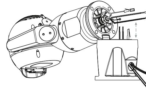
5. Carefully tilt camera to side with pin under hook.
