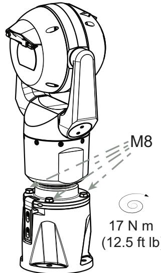
7. Carefully tip camera to final position. Avoid pinching wires between camera base and DCA! Insert four washers and hex bolts (supplied).
