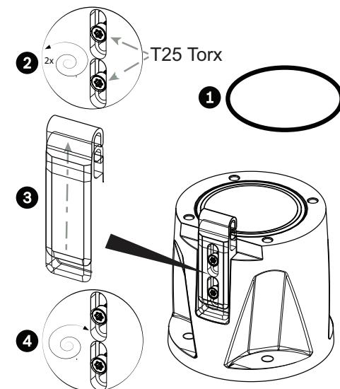
2. Insert O-ring (item 1). Loosen Torx bolts two (2) turns (item 2). Slide hook up (item 3). Tighten bolts to hold hook in place temporarily (item 4).
