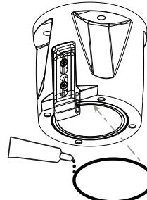
3. For inverted installation, apply a small amount of grease to primary O-ring to hold it in place.
