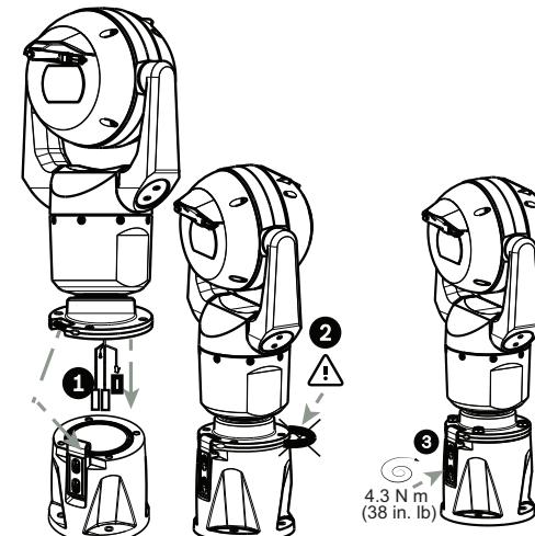
4. Place wires into DCA while positioning base pin of camera under hook (item 1). Avoid pinching wires! (item 2). Slide hook down to secure camera pin. Fully tighten hook bolts (item 3).
