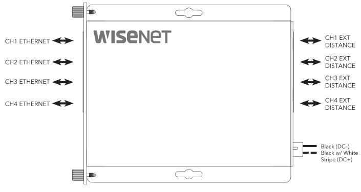
Operating Power: 9 to 15 VDC Power Consumption: 5W
