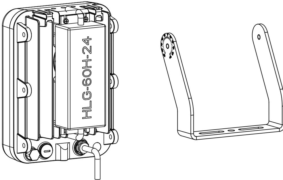
2. Secure the B03 bracket to the preferred mounting position.
