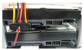
4. Place the HDDs inside the DVR, screw the HDDs from the bottom side of the DVR using the supplied Screws.
