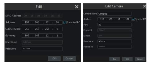
Click to edit the added camera as shown on the above right. Enter the new camera name, IP address, port, username and the password of the camera. You can click "Test" to test the effectiveness of the input information. Click "OK" to save the settings. You can change the IP camera name only when the added camera is online. Click "Next" to continue.
