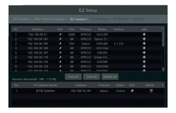
Click of the searched IP camera as shown on the below left. Enter the new IP address, subnet mask, gateway, username and the password of the camera. You can check "Sync to IPC" to modify the IP address of the IPC via different network segments for being in the same network segment with the NVR. Click "OK" to save the settings.
