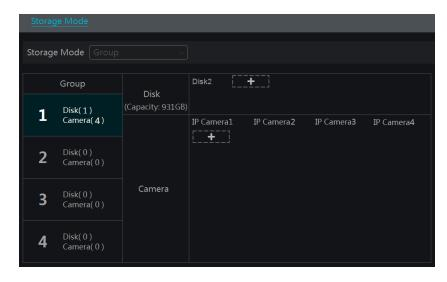
There are all four disk groups. By using disk group, you can correspond the camera to disk (the record data of the camera in the group will be stored into the disks in the same group). The NVR with e-SATA interface supports e-SATA recording.
