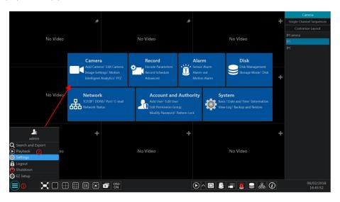
The setup panel includes seven modules. Each module provides some function entries with links for convenient operation.
