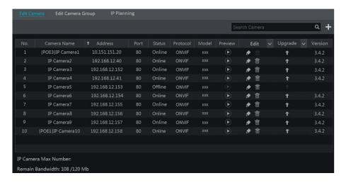
The IP cameras with PoE function which directly connect to the PoE port of the NVR will be displayed automatically in the camera list. Refer to the picture below. The IP camera which occupies the PoE resource has a prefix shown before its camera name. The prefix consists of PoE plus PoE port number. The IP camera which connects to the PoE port cannot be deleted from the camera list manually.
