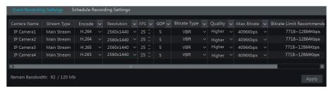
Click Start -> Settings -> Record -> Stream Settings to go to "Sub-stream" interface. Set the encode, resolution, FPS, GOP, bitrate type, quality and max bitrate of sub-stream for each camera in the interface and then click "Apply" to save the settings.
