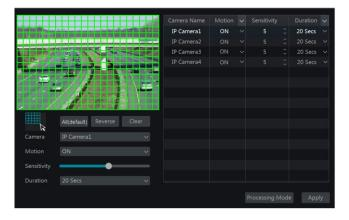
② Select the camera, enable the motion and set the sensitivity and duration of the camera.
