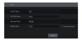
HTTP Port: the default HTTP port of the NVR is 80. The port number can be changed to others like 81. The port is mainly used to IE remote access. If you want to access the NVR through IE, you should enter IP address plus HTTP port in the IE address bar like http://192.168.11.61:81.
